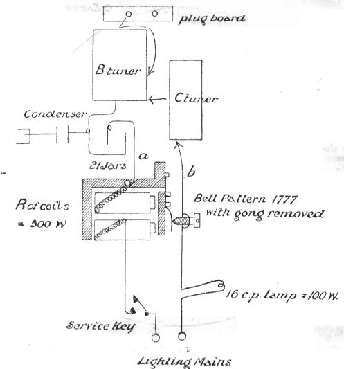
The make-and-break of buzzer takes the place of the spark gap in the ordinary
